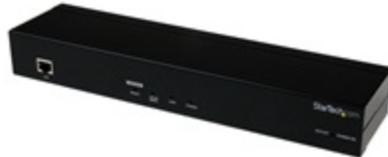
The SV1108IPPWGB 1 Port Remote Control IP KVM Switch with IP Power Control and Virtual Media lets you control a USB or PS/2 server remotely over a LAN or the Internet, and access the remote power switch feature to power on and off as necessary.
