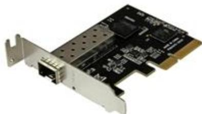
The PEX10000SFP 10 Gigabit Fiber Network Card is a cost-effective solution that delivers fast and reliable 10 Gbps network access at longer distances than copper-based networks. Using the SFP+ transceiver of your choice, you can connect your PCI Express-based server or workstation directly to your 10G fiber optic network.
