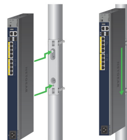
Attaching the Switch to a Round Pole
