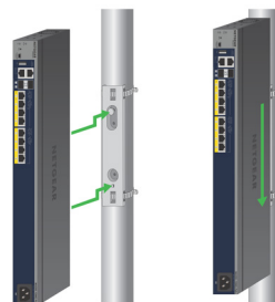
Attaching the Switch to a Round Pole
