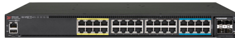
Brocade ICX 7450-32ZP 24×10/100/1000 Mbps RJ-45 ports and 8×100/1000 Mbps/2.5 Gbps RJ-45 ports with PoE/PoE+ support and 8 pre-assigned ports supporting PoH (95 W)
