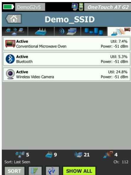
Figure 15. Unique Interferer analysis classifies sources of non-802.11
