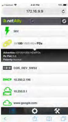
LinkSprinter Configured to test at 1 Gbps, but can only connect at 100
