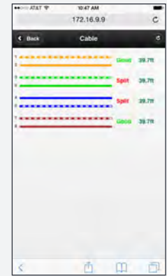
Split Pair detected with cable length to open
