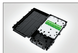
Inside view of MCCE with tray and 6 LC/APC Duplex Adaptors.
