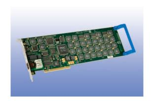
The PRI/E1-30 enables one server to support up to thirty concurrent communications with a mix of ISDN devices, V.90 modems, GSM mobile phones, and fax machines, making it an excellent choice for medium to large businesses. Because it is based on open-systems architecture, most industry-leading fax, unified messaging, computer telephony integration (CTI), and Voice over IP (VoIP) applications integrate easily when the PRI/E1-30 is used.
