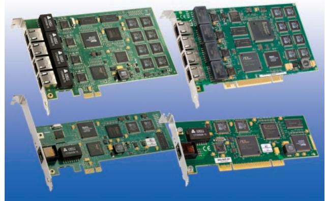
The Diva BRI offer voice, speech, conferencing, VoIP, modem and fax features, and can serve as a base for many communication applications. The boards support most standard applications, and are also suitable for new application development. The Diva BRI are available in Low Profile or Half Size form factors. The Diva BRI can be seamlessly combined with other Dialogic® Diva® Media Boards, such as analog, E1/T1, ISDN PRI, and VoIP.
