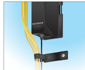
Strap the cables to the wall
