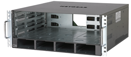
FRONT: Base chassis without blank panels
